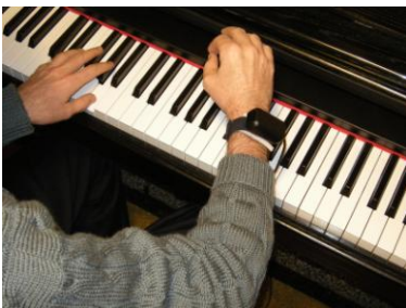
Right hand wearing tilt sensor from the Ricchetti Hyperviolin
